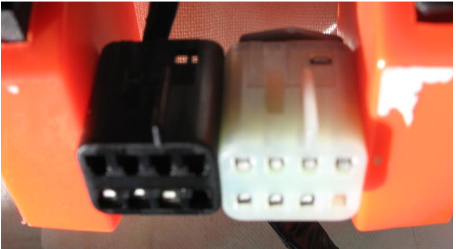
2012 Camaro Outside Mirror Connectors - Driver's Side Shown Black - Unheated • White - Heated • Same Exact Size
