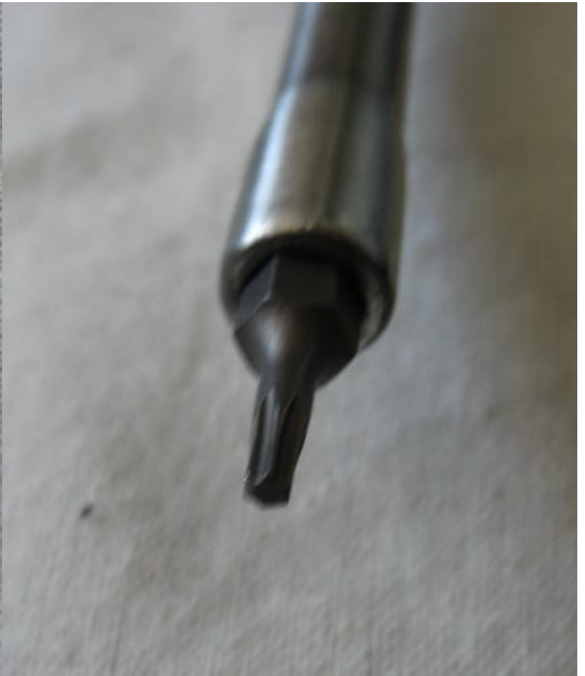
Using a Torx T-10 bit, remove the 3 screws holding the mirror motor in the mirror assembly.
