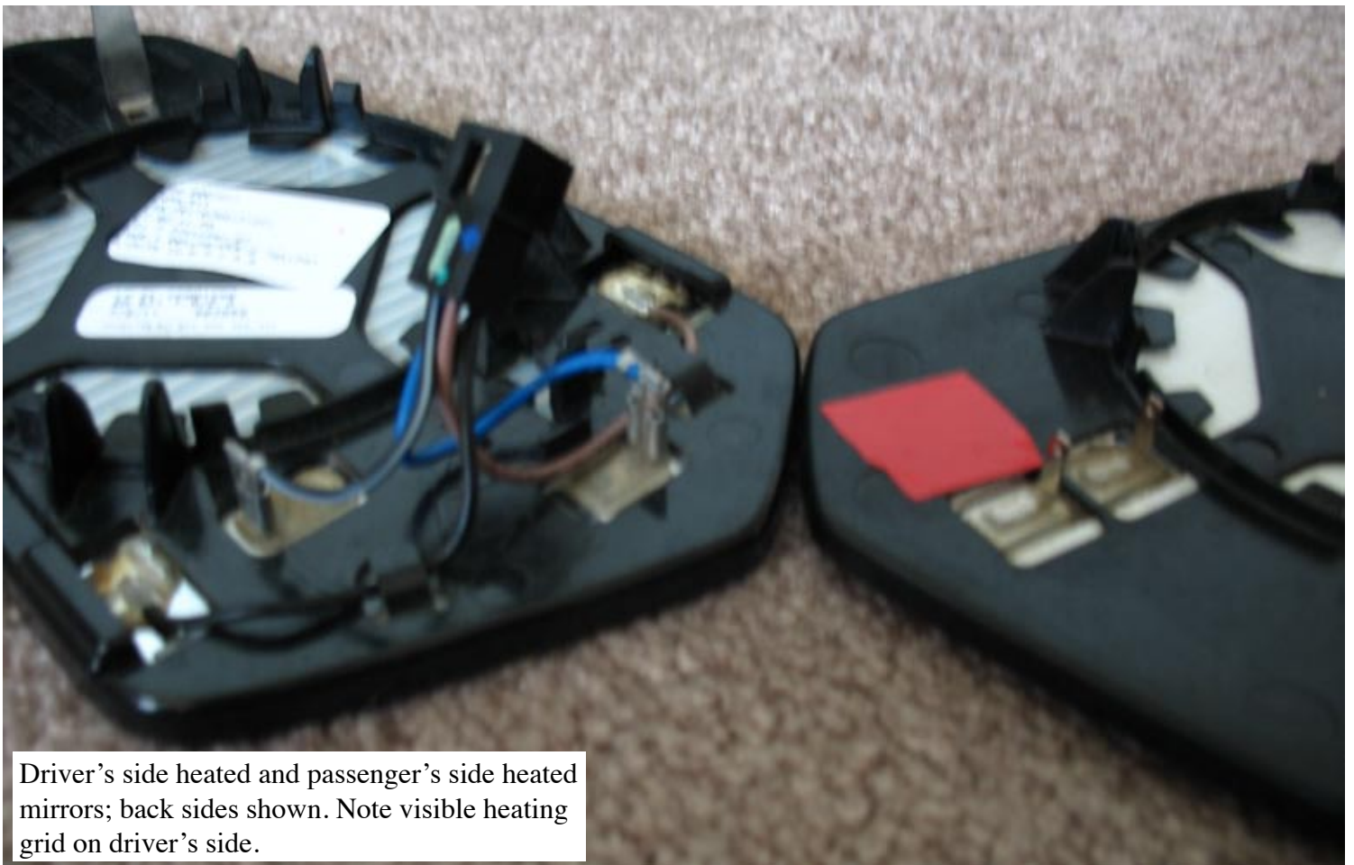
Driver's and passenger's heated mirror assemblies - completely disassembled. Note yellow and white wiring labels.
